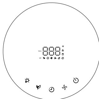
**UV indicator:** UV The indicator icon lights up and the UV mode is turned on.
