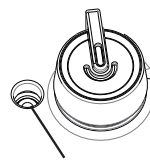
Unpressurized state (The float valve has fallen)
