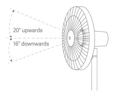
Gently lift or push down the fan's head or fan grille to adjust the airflow upwards or downwards.
