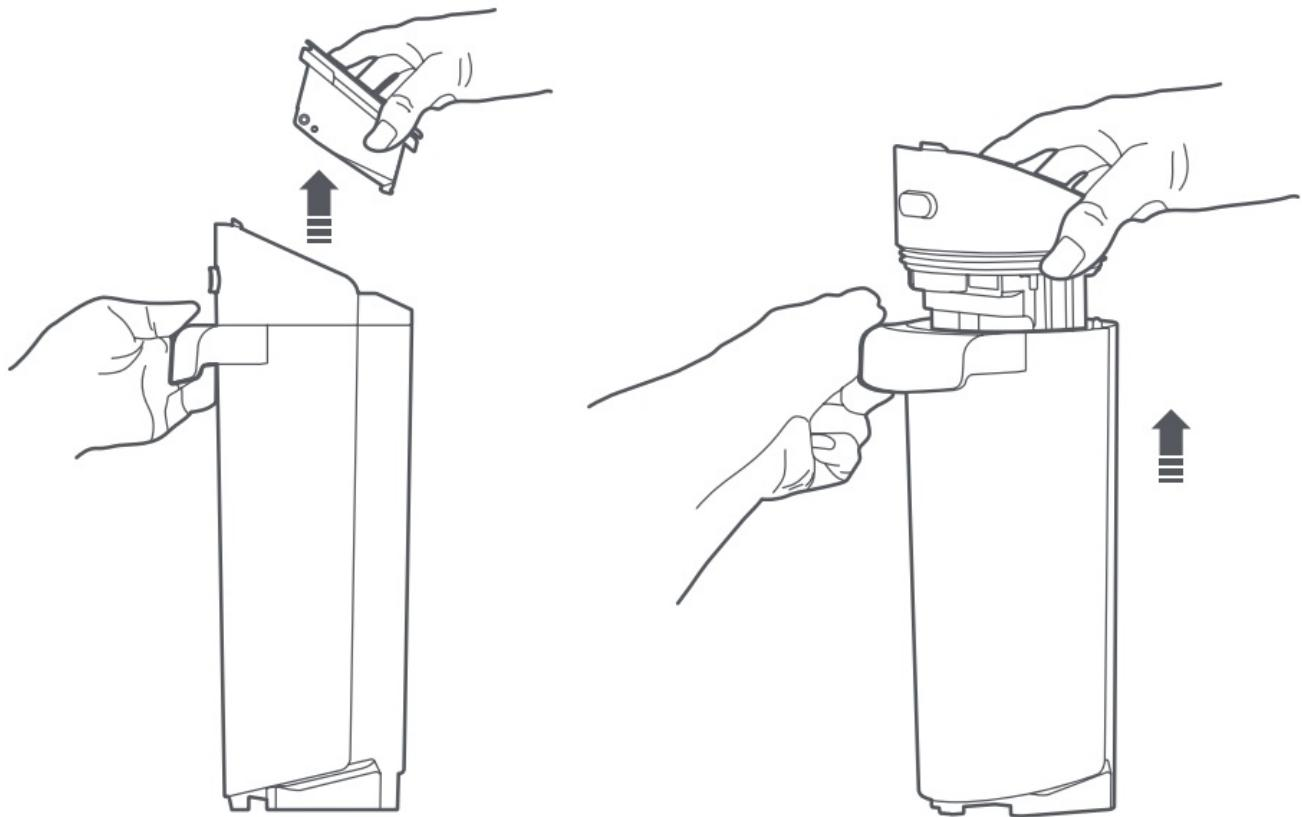
3. Press the dirty water tank release button to empty the dust compartment.
