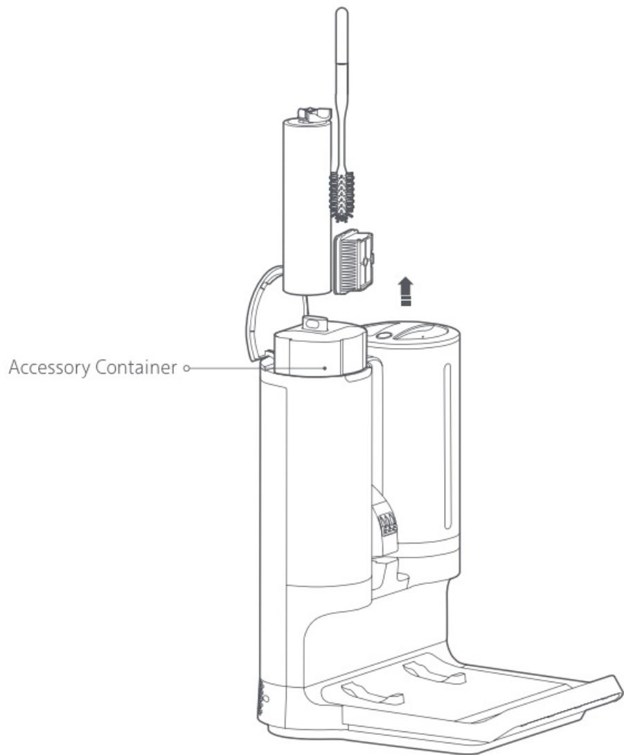
2. Clean the accessory container under tap water with the cleaning brush until the container is clean.
