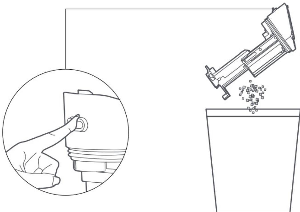
4. Rinse the dirty water tank, the dust compartment, and the filter with tap water until they are clean.
