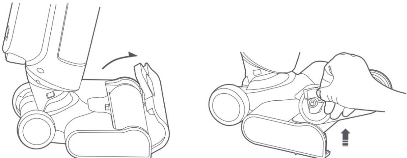
2. Rotate the handle of the cleaning brush to remove the blade. Use the blade to cut the hair tangled on the roller brushbar.
