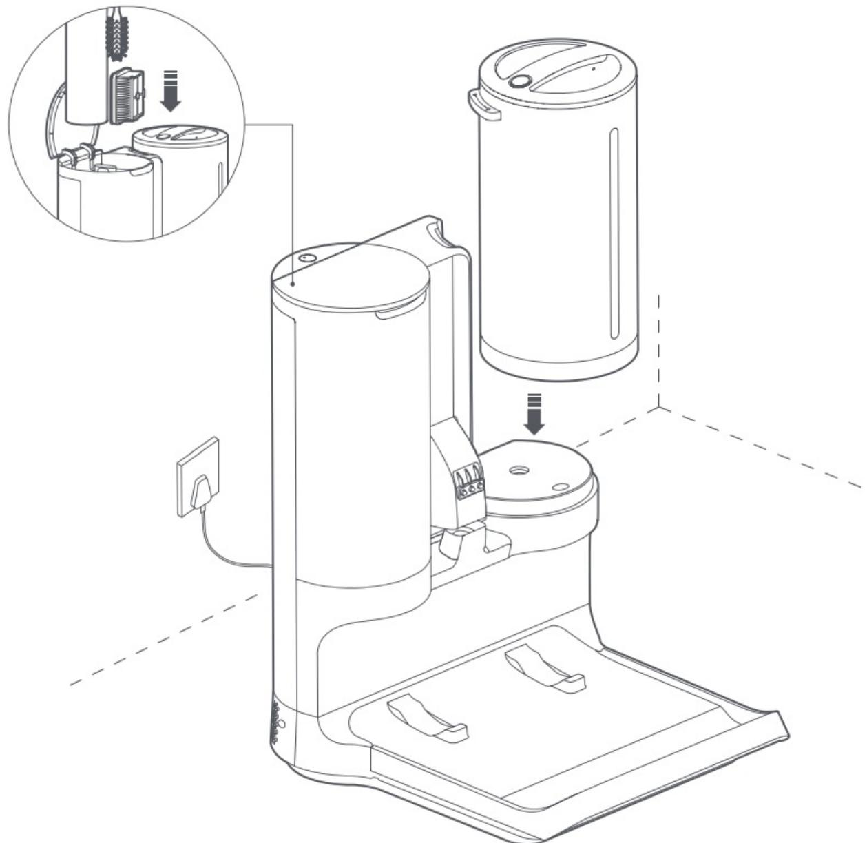
4. After the base station is powered on, place the vacuum on it to charge.
