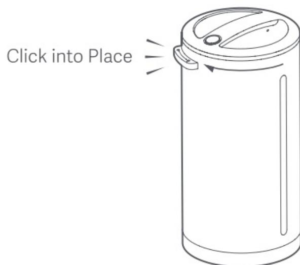
3. Put the water tank onto the base station. Open the accessory compartment, and place the spare roller brushbar, the spare filter, and the cleaning brush into the compartment.
