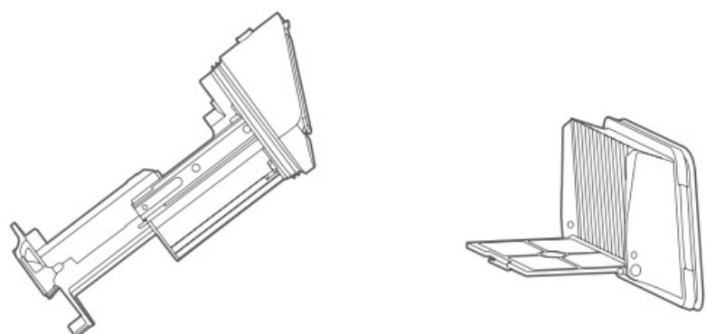
5. Put the cleaned filter into the accessory compartment, and close the compartment. Then press the accessory drying button to dry the filter.
