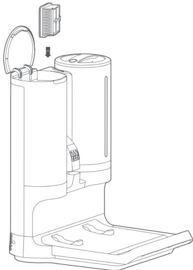
6. Install the dust compartment and a dry filter, and put the dirty water tank back into the vacuum in place.
